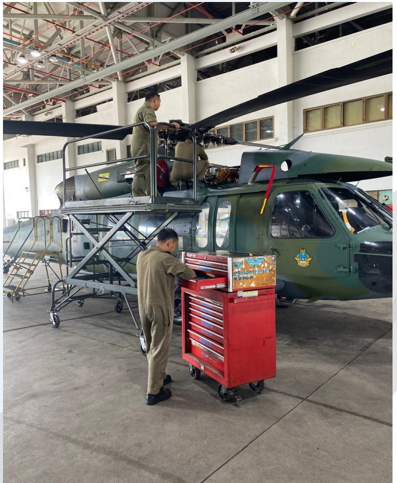
The correct practice of using the platform with safety fence when working at height.
